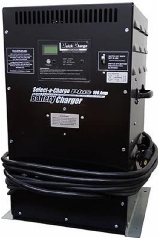
This model has a changeover tap to accommodate 208 or 230/240 volt input. You must check that your incoming power to the charger matches where the changeover tap is placed for the charger to work correctly. Always use a qualified electrician to install correct AC connections.
